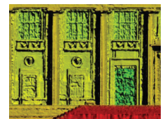
Facade digital surface model GeoTiff (.tif)
